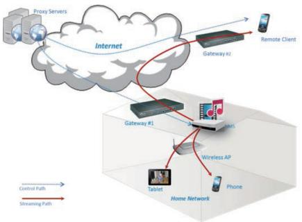
The RealHome Media Proxy is based on a Web API to provide a search engine-like user experience. Users can send the name of the specified home server to the Proxy and it will redirect to the relevant IP address.
