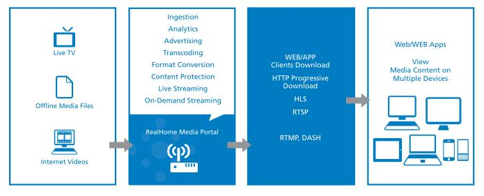
Similar to traditional OTT head-end software deployed in an Internet data center or back-end office, RealHome Media Portal offers these key capabilities:
