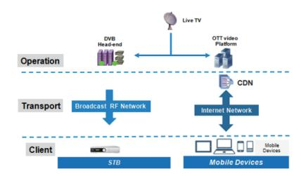
With RealHome Media Portal, set-top boxes become mini OTT head-ends so as to offload data traffic from mobile devices by leveraging set-top boxes' hardware capability. Therefore, operational costs are easily transferred to subscribers. Existing DVB billing systems can be used to charge on both DVB (digital video broadcasting) and OTT video services.
